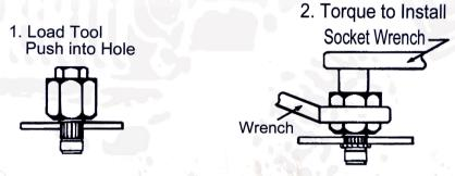
3. To Remove Tool: Torque Wrench opposite direction until tool disengages.
