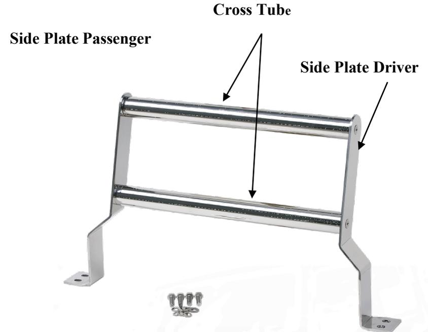
Place cross tubes in place on the side plates, fasten using the 82 Degree countersunk head bolts provided and tighten all four bolts.
