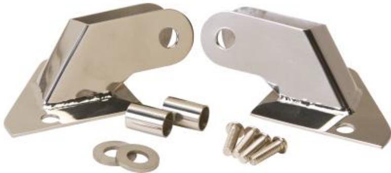
With Help remove the two bolts from the front side of the windshield hinge lower portion. Install the relocation bracket over the lower half of the windshield hinge and bolt in place using the stainless bolts provided. Remove the nut from the bottom of the factory mirror, then remove the spring and washer. Install the mirror into the bracket with the spacer between tabs. Install the factory washer and nut, then adjust the mirror and tighten securely.
