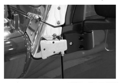
Carefully remove the two bolts on the lower part of the windshield hinge. Position and mount the relocation bracket using the 5/16" bolts provided. Remove the factory mirror from the door and mount the mirror to the bracket using ."-20nc bolts and nuts provided. Make sure all bolts are securely tightened. With help adjust the mirrors to your needs. We recommend that you use anti sieze on all threads of the stainless bolts provided with your parts.
