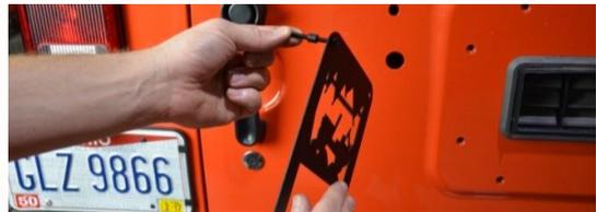
Tighten with a Phillips screwdriver. **DO NOT OVERTIGHTEN.**
