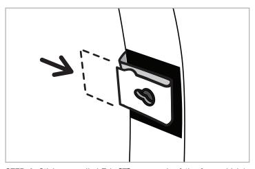
**STEP 4:** Stick a supplied Tab **[F]** over each of the four vehicle's factory holes, and wrap Tabs around the metal lip. Then, slide a S-clip **[G]** over each Tab.
