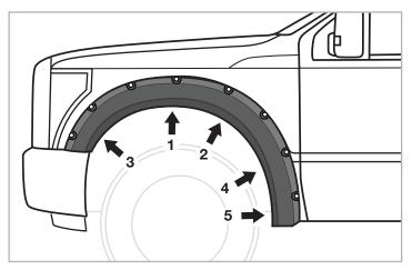
**STEP 2:** Hold flare in position, and reinstall the 5 factory screws through holes in flare and into vehicle's factory holes in the order indicated above.
