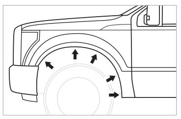
**STEP 1:** With a 7/32" socket wrench, remove 5 factory screws and keep for later use.
