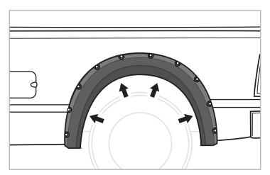
**STEP 3:** Hold flare in position, and ensure holes in flare aligns up with vehicle's factory holes.
