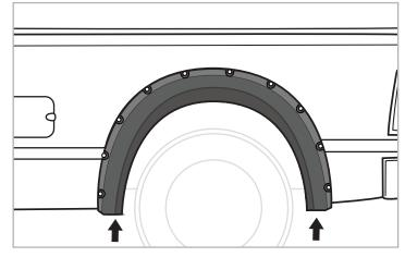
**STEP 6:** With a 5/32" Allen Wrench and 3/8" socket, install a supplied Bolt **[I]**, Washer **[J]**, Spacer **[K]**, Washer **[L]**, and Nut **[M]** through bottom 2 holes in flare and into vehicle's factory holes. Refer to Fig 3.
