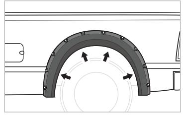
**STEP 5:** Reposition flare. With a #2 Phillips Screwdriver, install 4 supplied PH Metal Screws **[H]** through holes in flare and into S-clips staring with top two locations.
