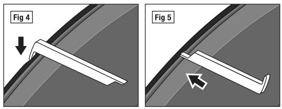
**STEP 7:** If needed use supplied tool **[N]** to trim outer edge (Fig 4) and inner edge (Fig 5) by inserting tool ends then sliding around the entire edge trims from one end to the other as shown in above pictures.
