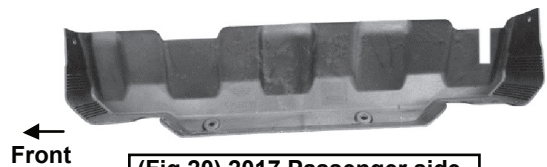
(Fig 20) 2017 Passenger side DEF cut for example only
