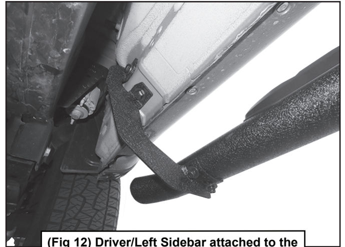
(Fig 12) Driver/Left Sidebar attached to the Rear Mounting Bracket
