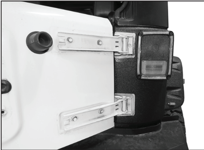
(Fig 4) Remove covers from hinges and around hinge anchors. Remove hex bolts attaching hinges to door. Remove rear door
