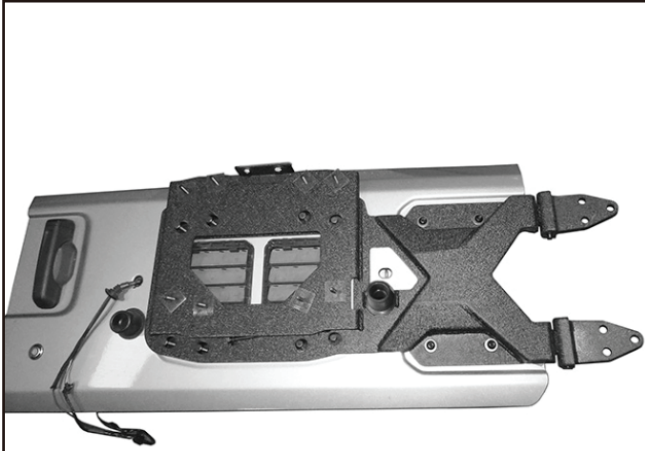
(Fig 12) Mount assembly attached to tailgate. Reuse factory screws to attach tailgate assembly to vehicle. Reattach check rod and passenger side plastic cover
