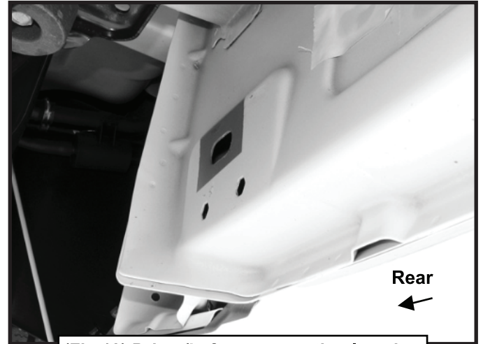
(Fig 13) Driver/Left rear mounting location
