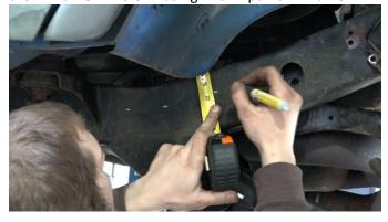
Using a tape measure, measure in from the front body mount bracket 1.5 inches and make a mark using a paint marker.
