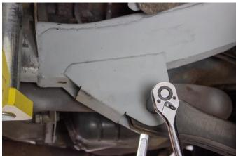
Reinstall upper control arm using 17mm socket.
