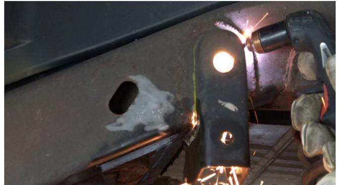
Begin cutting away the track bar bracket as close to the frame rails as possible.
