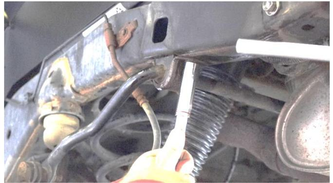
With an 18mm socket, remove the body mount bolt and bushing and set it aside to be reused later.
