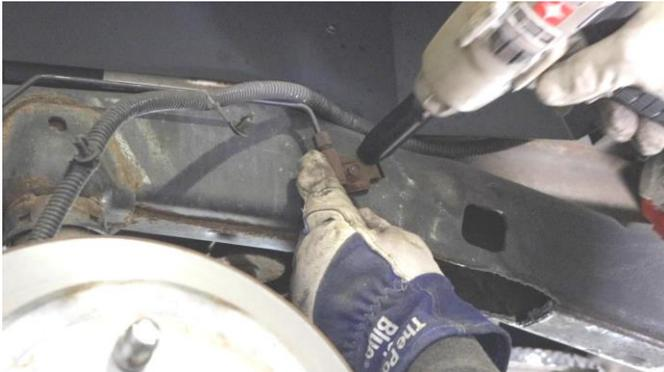
With a 22mm socket, remove the bolt securing your track bar and push it down and out of the way.
