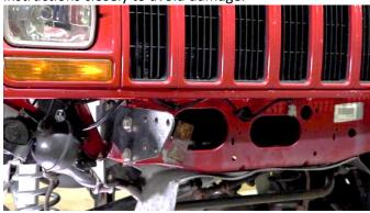
With a 10mm socket remove the retaining bolt of the fender support bracket. You will then need to pull the bracket away slightly in order to slide the stiffener into place.
