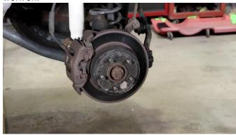
With a T40 Torx, Remove the bolt from the break line retaining bracket, and remove the body clips of the rearmost inner liner with a body clip remover.
