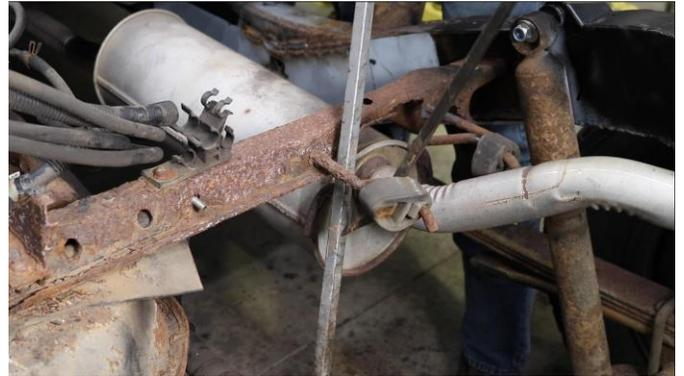
With a 13mm socket, remove the bolt retaining the gas tank strap, and set it aside if not replacing it.
