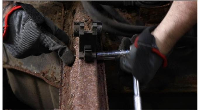
With a 13mm socket and wrench, remove the 4 bolts from each frame rail, freeing the crossmember. Remove the crossmember.
