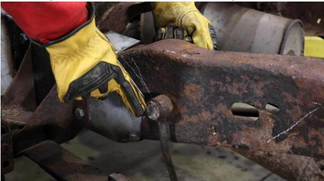
Hold the part up to the frame using the frame holes for alignment and take note of its coverage. Mark off any sections you wish to cut off, while leaving enough to weld back on to.
