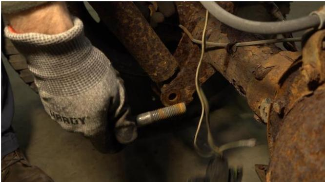
Begin punching out the rivets retaining the rear spring hanger. Support the vehicle and lower the axle. Remove the rear crossmember bolt from the bottom of the rail.
