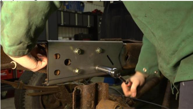
Remove any potential fire hazards from the work area. Tac weld the part to the frame. Following proper welding procedures, begin welding the part.
