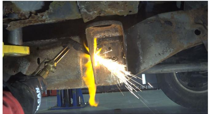
Clean the frame free of rust and debris, revealing bare metal, while leaving enough material to weld back onto.
