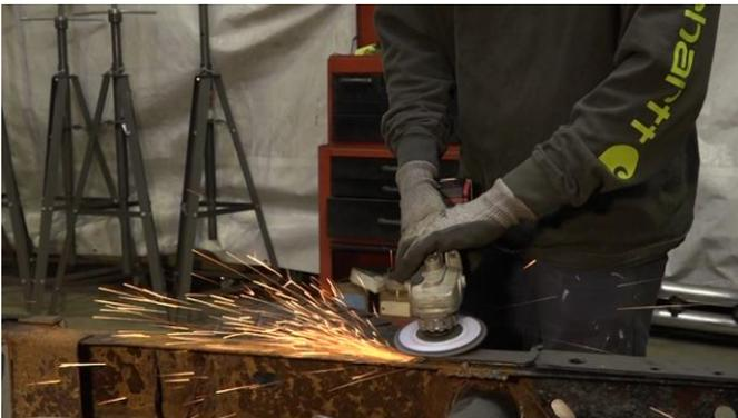
(OPTIONAL) Paint the part and work area with a weldable primer to help prevent against rust. By either referencing the opposite side by taking critical measurements (distances from frame holes, slots, etc.), or by using a flat, weld-safe section such as a plate or tubing, line up and clamp the mount
