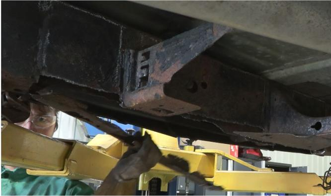
While cutting the crossmember wings, ensure you leave enough material to weld back onto the frame section.
