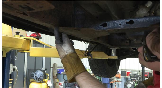
Additionally, the wings on the transmission crossmember will need to be cut in order for the part to slip on.
