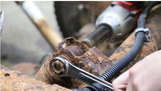
After the shock has been disconnected, begin removing your rear spring hanger with your cutting wheel or torch by cutting off and prying out its rivets.
