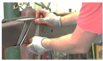
Following proper welding procedures, start by welding the front end of the crossmember into place.
