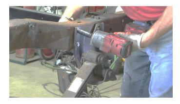
Remove the bolts on the top and bottom of the frame holding the crossmember in place.
