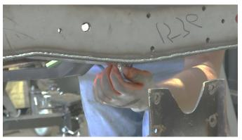
Reinstall your leaf spring hanger using a 14mm socket for the bolts and a 15mm socket for the nuts.
