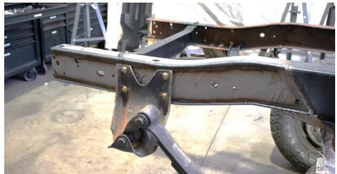
Reinstall your leaf spring hanger using a 14mm socket for the bolts and a 15mm socket for the nuts.
