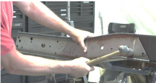
Following proper welding procedures, start by welding the front end of the crossmember into place.
