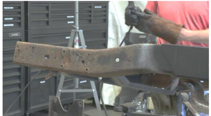
Remove the bolt on the bottom of the frame holding the crossmember in place.
