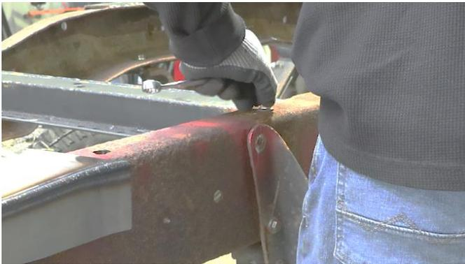
Our part features eight perforated plates on the top and bottom of our frame section to fit over the rivets retaining the factory center frame crossmember. If you decide to keep your rivets, cut out the perforated plates.
