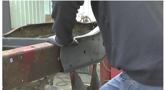
If you installed our center frame crossmember (RB7363), use a 14mm socket and 15mm wrench to install the eight bolts on the top and bottom of your frame rail to hold your crossmember and leaf spring frame section in place.
