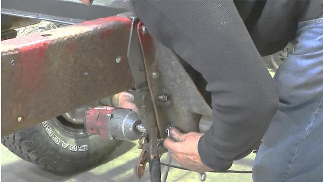
Following proper welding procedures, tac weld your leaf spring frame section onto the frame before welding it on fully. Weld 100% around all edges.
