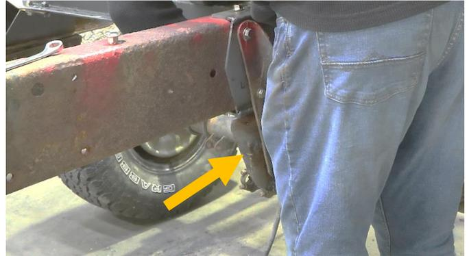
To align the leaf spring hanger with the 4WD and heavy-duty bracket, we will need to make some slight adjustments. To do this, we recommend lining up the bracket and leaf spring hangers' holes to the best of your ability. Then, using a torch, burn your way through the holes so the bolts will align properly.
