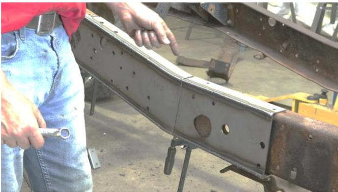
Slide the part onto the frame using the frame holes to help with the alignment. Use a hammer to push it into place.
