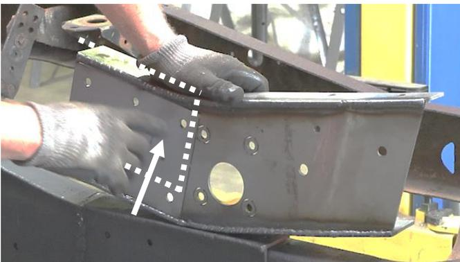
Our part also features 4 small perforated plates that you can remove to fit over any existing rivets you may have on your frame.
