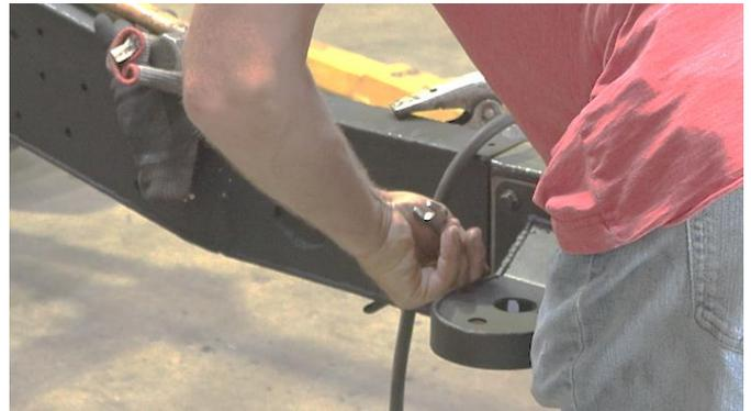
Weld the part on fully. 100% around all edges.
