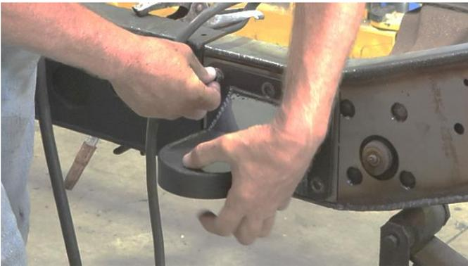
Following proper welding procedures, tack weld the front end of your frame section onto the frame, leaving the side with your body mount loose.
