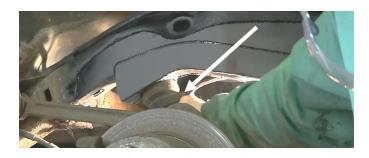
To hold your bump stop in place, you'll need to punch down the tabs located inside the frame section. Set your punch above the spring and using a hammer, punch down the tabs.
