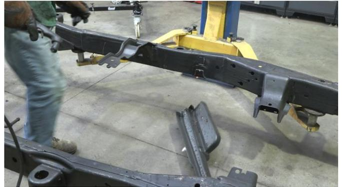
After you have successfully removed the OEM Front Frame Support Crossmember, use your hand grinder to clean the areas of the frame where the crossmember was previously attached. Remove all rust possible, as you will need to create a smooth and clean point at which you can attach your replacement crossmember.
