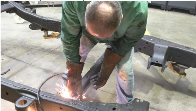
Once both sides have been thoroughly cut, the crossmember should come free of the frame rails with little to no difficulty.
