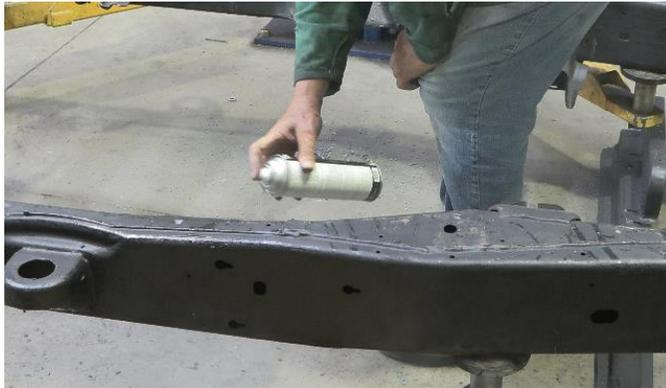
Additionally, the primer will set the base on which the crossmember can be sufficiently welded.
