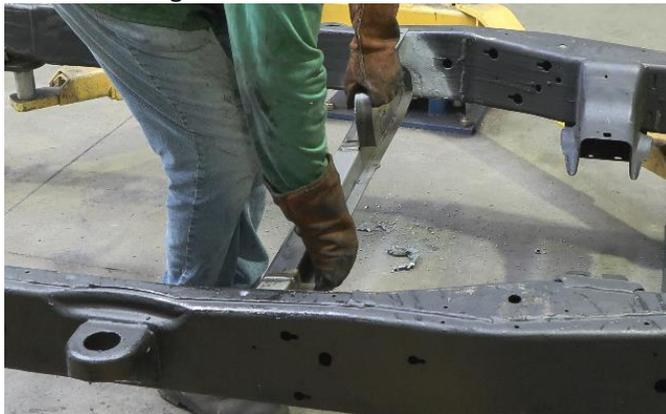
required tools and equipment, slide the front frame support crossmember into place, one side at a time.
