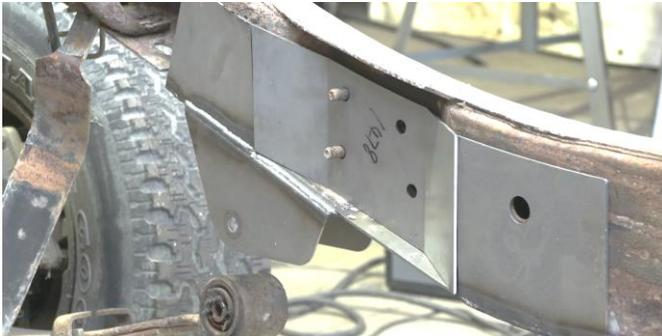
Hold the fuel tank bracket up to the frame and using a 15mm socket, screw the 4 nuts into place.
