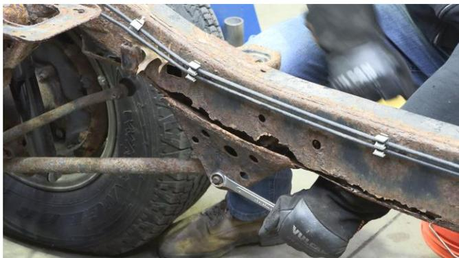
Hold the part up to the frame and mark off the part's cutline  $\frac{3}{4}$  inch from the bottom of the frame.
