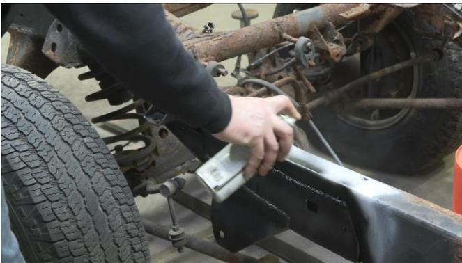
Then, reinstall the lower control arm bolt with a 19mm socket.
