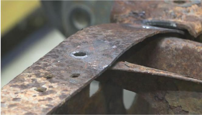
Grind away any remaining rust and debris revealing bare metal. Coat the part and work area with a weld-through primer to help prevent against further rust development. Followed by painting the part and work area with a weldable primer to help prevent against rust development.
