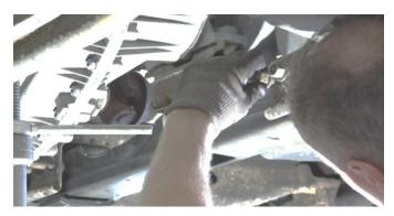
With a 7/8" socket, reinstall the bolts on each end of your crossmember.
