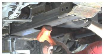
Insert a bolt on each end of the transmission crossmember to hold it in place. Then, lower your jack stand supporting the crossmember.
