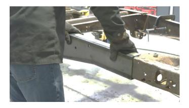
Following proper welding procedures, tac weld your over-axle frame section onto the frame before welding it on fully. Weld 100% around all edges.
