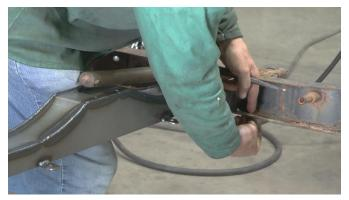
Using a 13mm socket, screw the support bars into place with the included M8 nuts and bolts.
