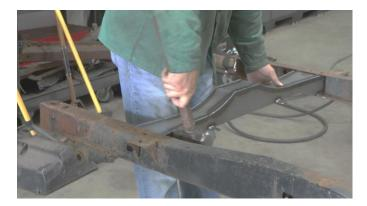
With a 13mm socket, install the M10 bolts. With a 15mm socket, install the M10 nuts. Repeat on both sides.
