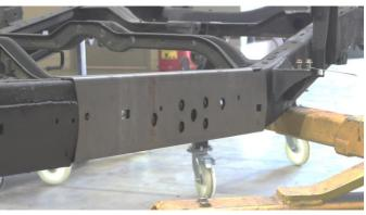
Following proper welding procedures, tac weld the center frame section onto the frame before welding the part on fully. Weld 100% around all edges.
