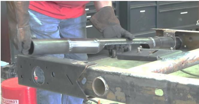
Following proper welding procedures, tack weld the crossmember to the spare tire plate before welding it on fully.
