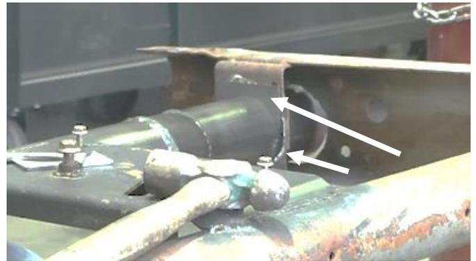
Our part features eight support plates to fit on the top and bottom of your inner brackets located on each end of your crossmember. Hold the plates up to the frame and tack them into place.
