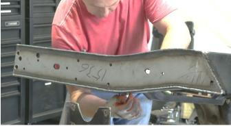
Reinstall your leaf spring hanger using a 14mm socket for the bolts and a 15mm socket for the nuts.
