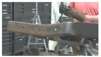
Remove the bolt on the bottom of the frame holding the crossmember in place.
