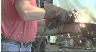
To ensure a tight fit, screw the two bolts on the end in with a 15mm socket before welding the rest of the frame section into place.
