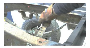
Spray the work area with a weld through primer to help prevent against rust development.
