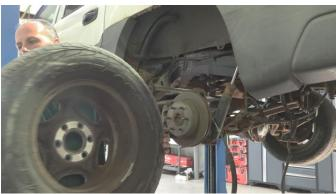
Using a 21mm socket, remove the bolt holding the shock in place.
