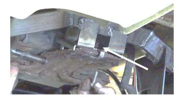
With the included hardware, reinstall your EVAP can with an 13mm socket.
