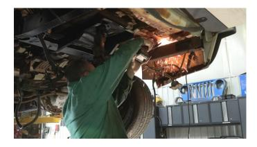
Coat the part and work area with a weldable primer to help prevent against rust development.
