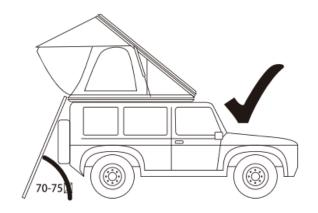
Once the tent is fixed securely to the vehicle's roof rack and the vehicle is positioned with the hand brake applied, attach the ladder, and ensure that it is secure and is locked in position and on an angle of 70 to 75 degrees.
