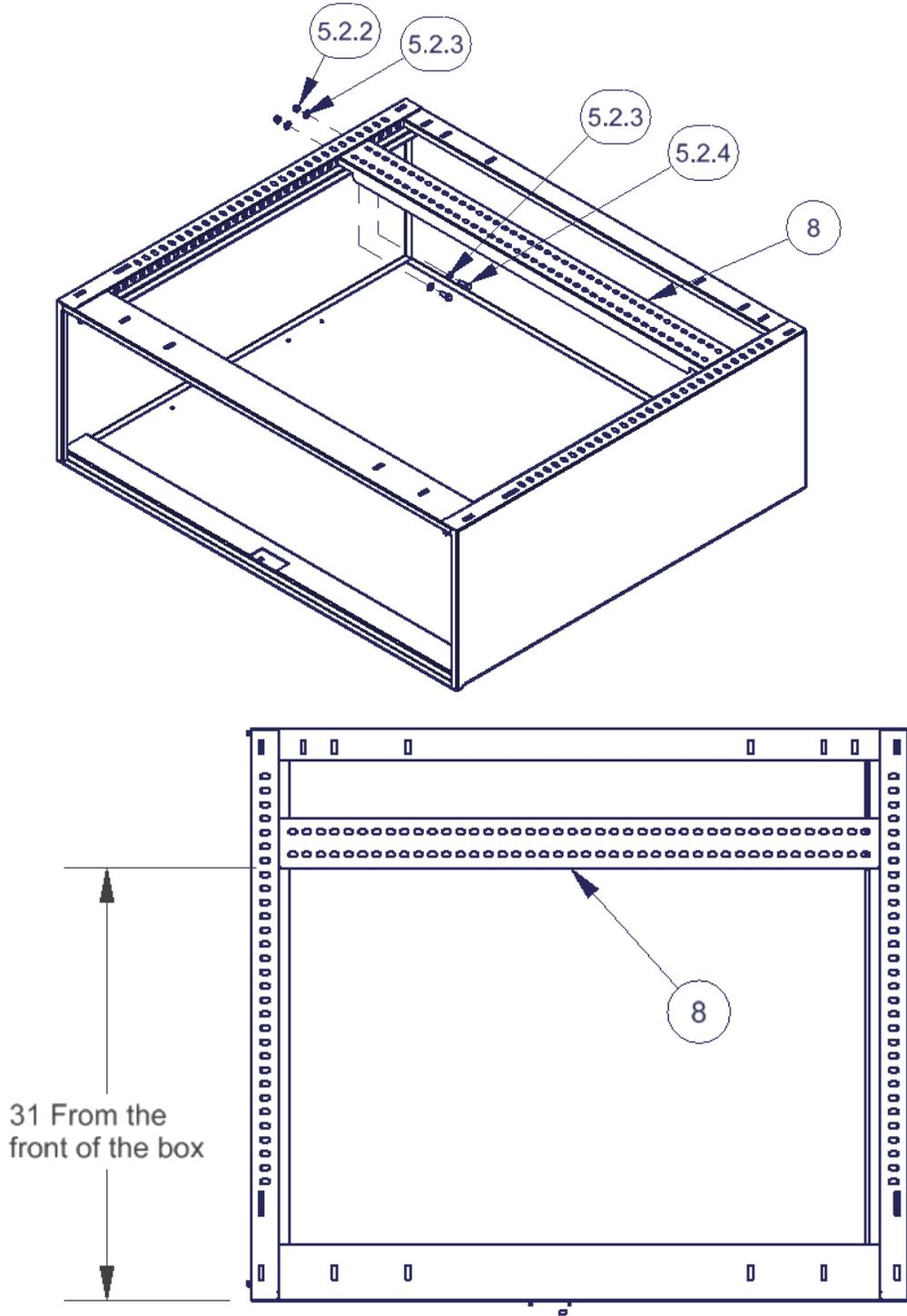
5. Assemble the mounting brackets as illustrated. Be sure left and right sides are assembled opposite. (See Figure 3)
