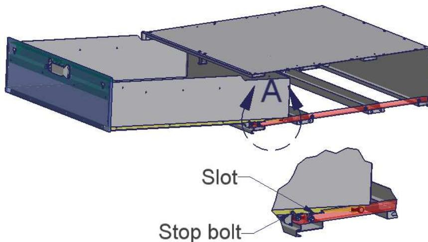
4. For a standard mounting application as described above fasten only (1) #8 mounting bracket to the drawer enclosure with the illustrated hardware. These bolts are difficult to reach; Use a ½" shallow socket with a long extension and a ratchet (Universal joint also helps) and a ½" wrench on the other end. Unbolting the slide using a 7/16" wrench will make things easier as well. **These parts and fasteners are included with the drawer.** (See Figure 2)
