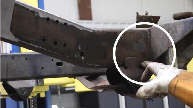
Begin measuring and trimming the stiffener to size.
