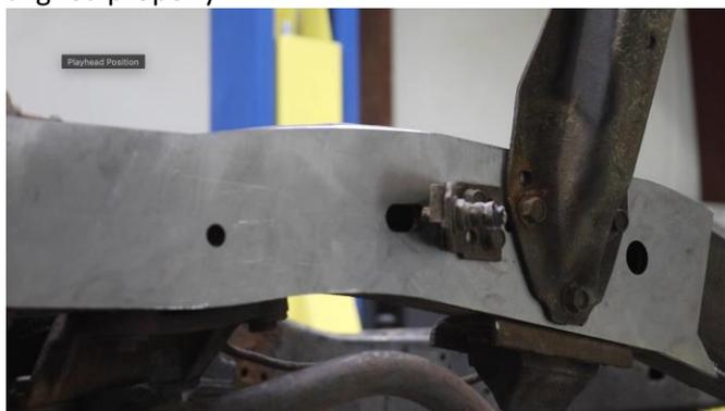
The second stiffener is made to be universal and must be trimmed to your vehicle's measurements.
