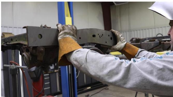
Begin cleaning the frame free of any rust and debris, revealing bare metal.
