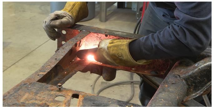
On C-channel parts, we only recommend cleaning the frame and removing thin areas in the frame as the part welds around the frame. Hold the part up to the frame and mark off its coverage to be cleaned.
