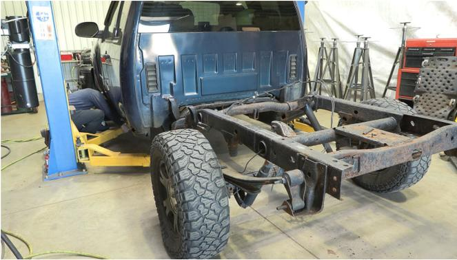
Unbolt the shock with a 21mm socket.
