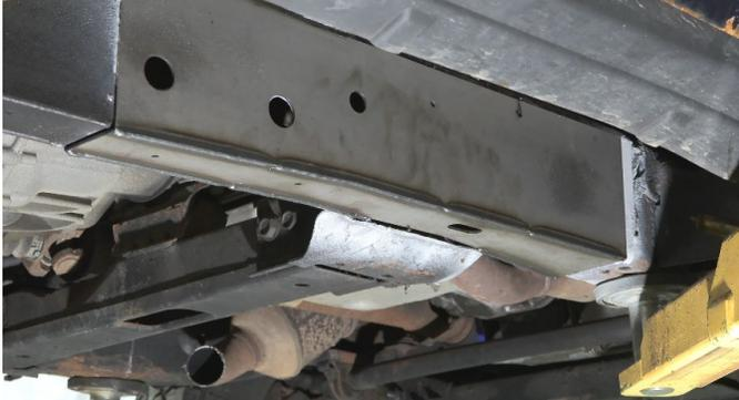
You will need to cut the flanges of the transmission crossmember for the part to slide on. Ensure that you cut them flush with the frame rail. This is important because you will need to weld them back onto the part, and if there isn't enough material, there will be a large gap.
