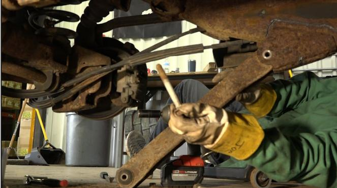
Hold the part up to the frame and take note of its coverage. Mark out a cut line at least 1 inch from the bottom of the frame and trailing arm mount. Ensure that you retain enough material to weld back on to.
