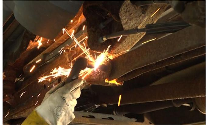
Grind away any remaining rust and debris revealing bare metal. Coat the part and work area with a weld-through primer to help prevent against further rust development. Followed by painting the part and work area with a weldable primer to help prevent against rust development.
